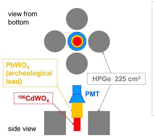
4 HPGe, ~ 225 cm<sup>3</sup> each, in one cryostat
