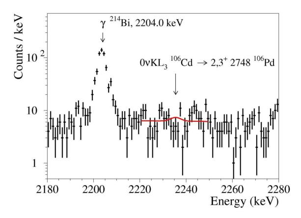
Sum energy spectrum of four HPGe detectors accumulated over 13085 h in region where the 2236 keV peak from deexcitation of 2748 keV excited level of <sup>106</sup>Pd is expected (possible resonant  $0_V KL_3$  electron capture).  $T_{1/2} \ge 8.7 \times 10^{20}$  yr at 90% C.L.
