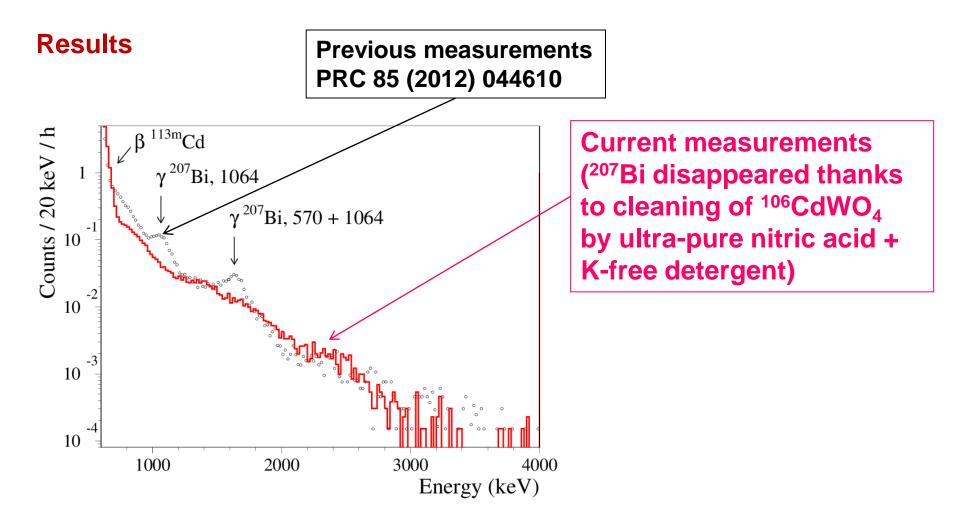
Spectrum of <sup>106</sup>CdWO<sub>4</sub> ( $\beta/\gamma$  events) measured during 13085 h (anticoincidence with HPGe) [F.A. Danevich et al., AIP CP 1549 (2013) 201]
