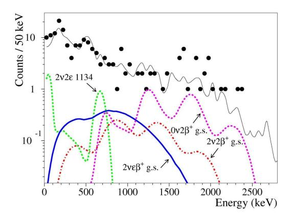
Energy spectrum of the <sup>106</sup>CdWO<sub>4</sub> detector accumulated over 13085 h in coincidence with 511 keV annihilation  $\gamma$  quanta at least in one of the HPGe detectors (circles).
