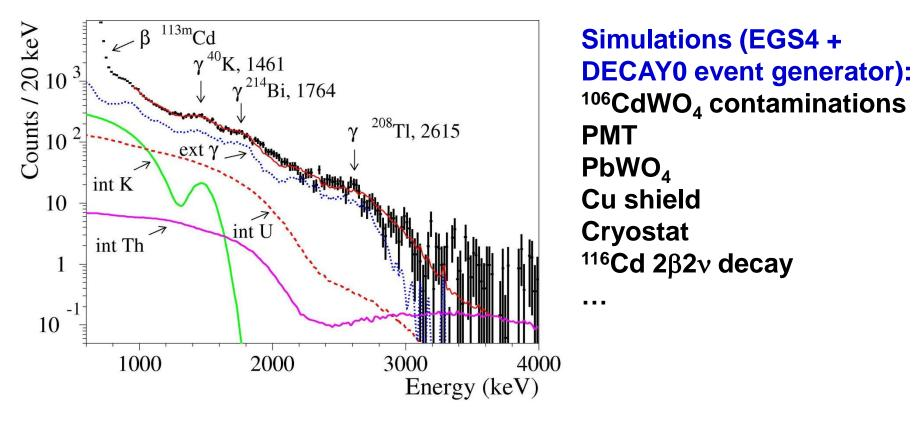
Energy spectrum of  $\gamma(\beta)$  events in <sup>106</sup>CdWO<sub>4</sub> accumulated over 13085 h (points) in anticoincidence with HPGe together with the background model (red continuous line).
