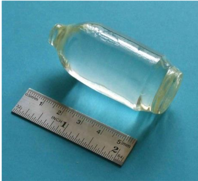
^{106}\text{CdWO}_4 crystal 231 g \delta(^{106}\text{Cd}) = 66\% yield of crystal = 87%
