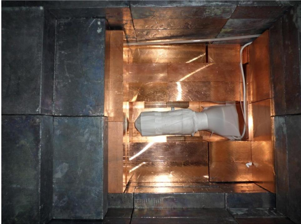
The  $\text{ZnWO}_4$  crystal scintillator **after the recrystallization** and the were viewed by a low-radioactive **3 in PMT** through a high purity **quartz light guide  $\varnothing 76 \times 100 \text{mm}$** .
