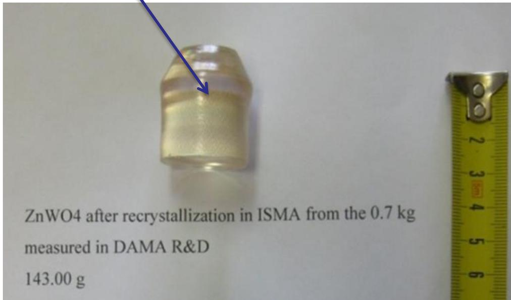
The side surface (~0.4 mm) layer of crystal was removed by fine grinding paper to check presence of radioactive contamination in external (surface) layer of the crystal.
