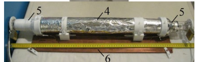
Photograph of the ^{106}\text{CdWO}_4 crystal scintillator (1) fixed by using poly(methyl methacrylate) support details (2) in polystyrene plastic light guide (3). Lower: quartz and plastic light guide (with the ^{106}\text{CdWO}_4 crystal scintillator inside), covered by aluminized foil (4), viewed by PMTs (5), assembled on a copper plate (6).
