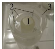
Schematic cross-sectional view of the experimental set-up used to measure ^{113\text{m}}\text{Cd} \beta spectrum in 2009. The ^{106}\text{CdWO}_4 crystal scintillator (1) is fixed in a cavity filled by silicon oil (2) inside polystyrene plastic light guide (3) and viewed through quartz light guides (4) by PMTs (5). The passive shield consisted of high-purity copper (6), lowradioactive lead (7), cadmium (8), polyethylene/paraffin (9), and a poly(methyl methacrylate) box flushed with \text{N}_2 gas (10).
